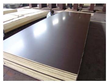
**Plywood** manufactured by pressing on standard plywood plate special paper impregnated with resin – so called film. Depending on the type of resin used to impregnate paper, we distinguish phenol films and melamine films. The process of pressing of the film runs in high temperatures and under high pressure. Resin from the film penetrates into wood giving the effect of a very tight bond with underlying plywood plate.
